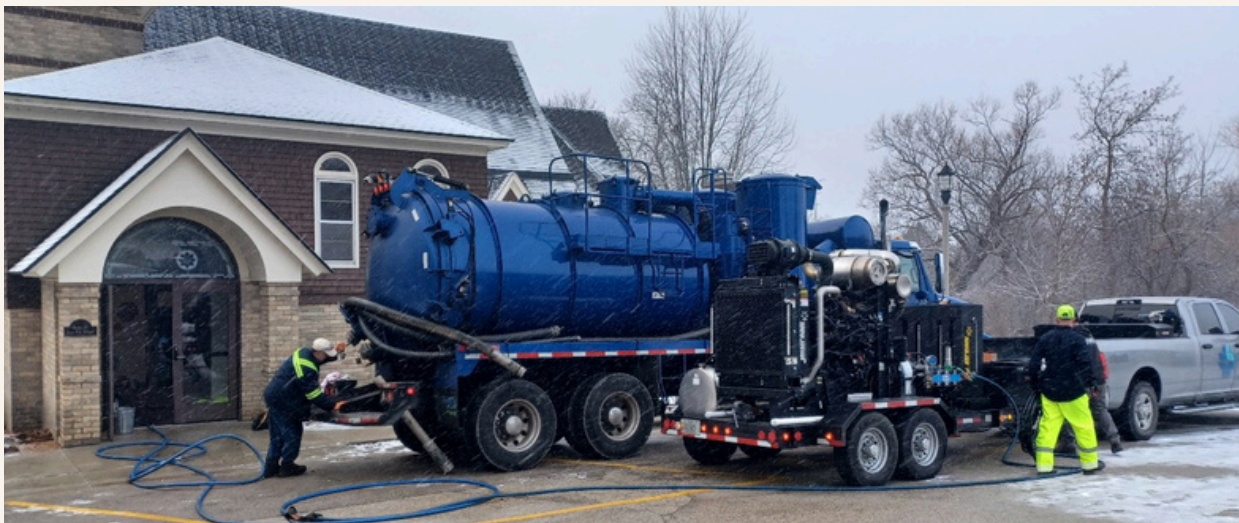
The blue 'Super Sucker' vacuum truck (in background) and the high-pressure water jet diesel pump trailer (in foreground)
